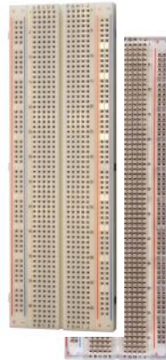
830-point breadboard with four power rails BB830™ - White BB830T™ - Transparent
